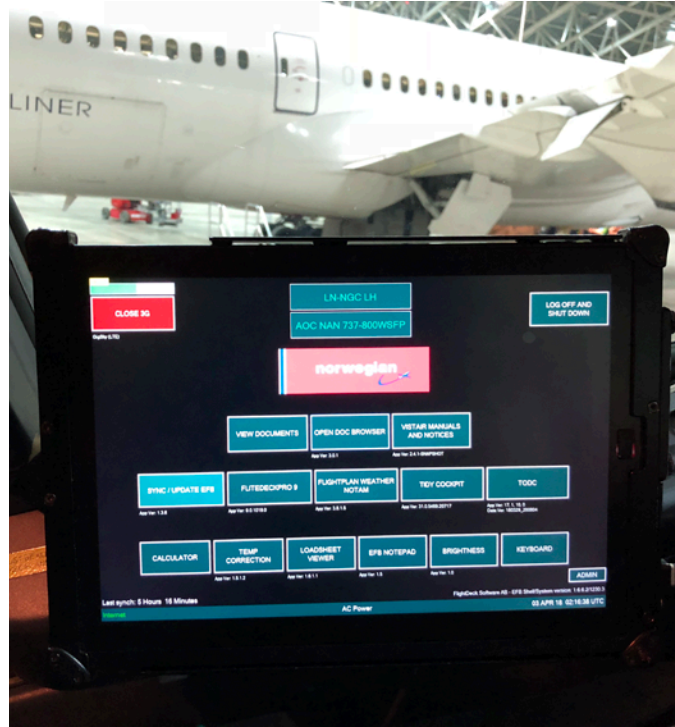
ThinkPad X1 Tablet being used as a Electronic Flight Bag (EFB) solution in the cockpit of a Norwegian flight
