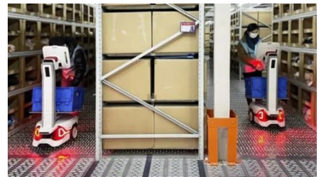
Order-to-Person Robots intelligently plan pick-up sequence based on the order task. Upon reaching the storage location, it guides the nearby workers to place the goods into the carrier.
