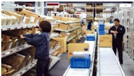
Person-to-Goods Workers run to each storage location to pick up items according to the order list and bring them to the shipping area.
